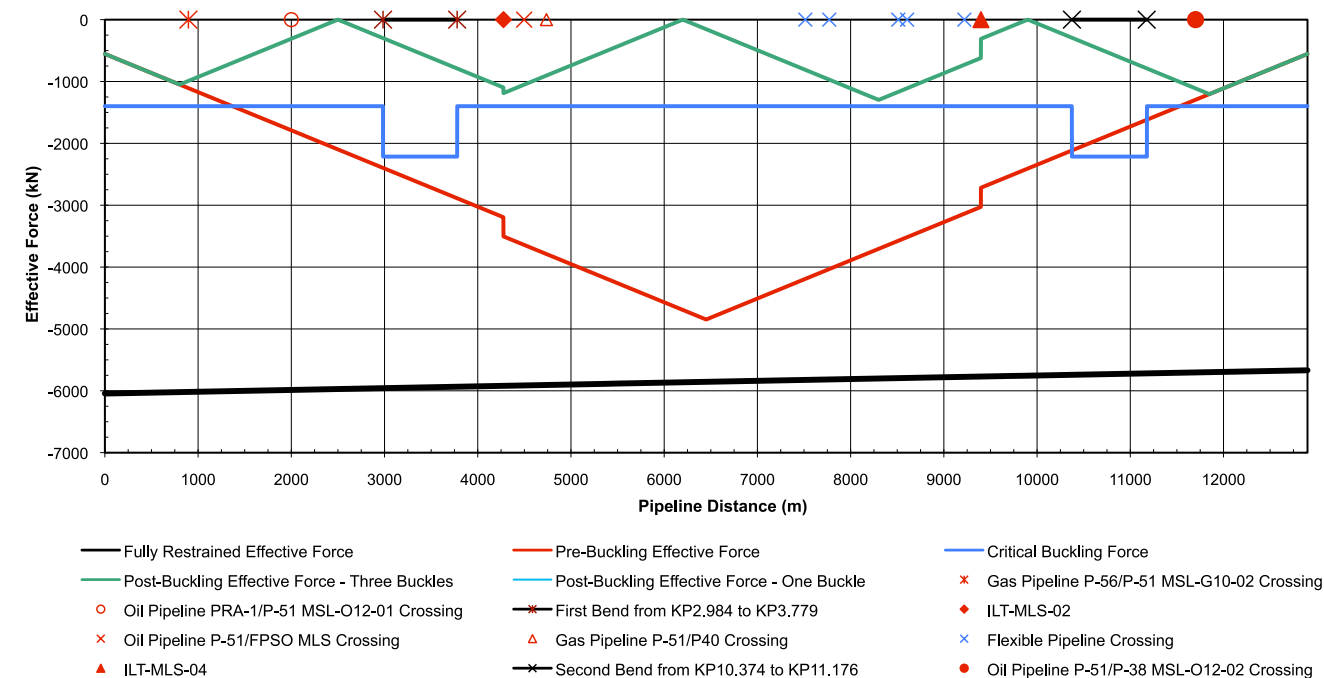
Figure 2: Effective Axial Force Profile (Base Case) and Locations of the Structures and Crossings
